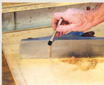
▲ Pic.6 Cleaning the mouth of the plane; MDF swarf is a real nuisance
